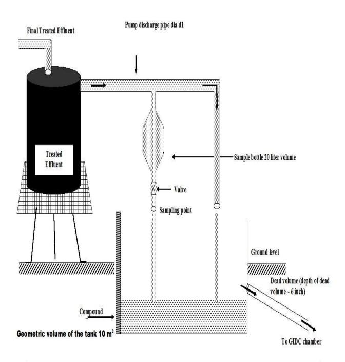
Note d1: Diameter of the discharge line should be such that it can not allow discharging the daily flow in a shorter duration say 2 – 3 hrs. Daily discharge strictly as per CCA, should take at least 18 – 22 hrs a day
